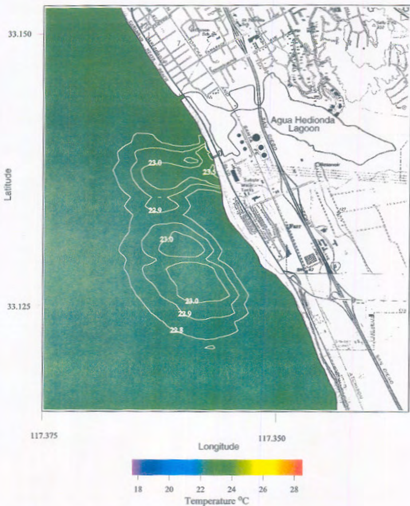
Figure 4.42. 30 day average of the depth-averaged temperature of concentrated seawater for R.O. = 50 mgd, plant inflow rate = 703 mgd, combined discharge = 653 mgd, ambient ocean temperature = 22.7 °C, worst month (August 1992).
