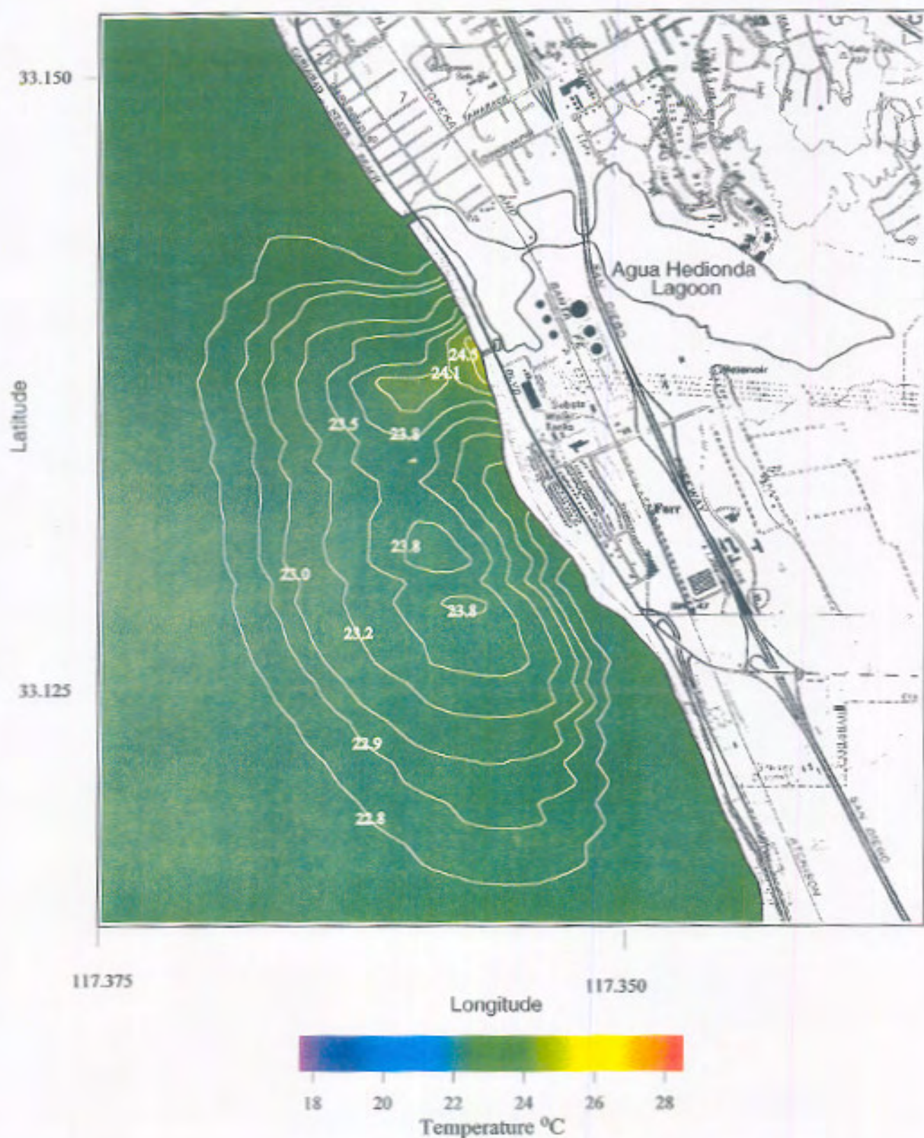
Figure 4.43. 30 day average of the bottom temperature of concentrated seawater for R.O. = 100 mgd, plant inflow rate = 703 mgd, combined discharge = 603 mgd, ambient ocean temperature = 22.7 °C, worst month (August 1992).
